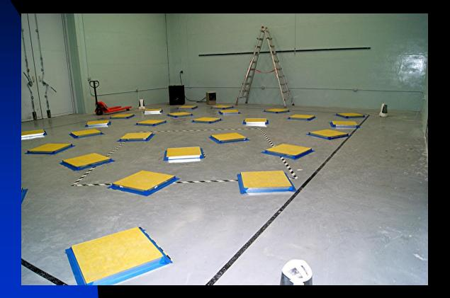
Test 3 was to test the idea that moving air might inflate the high frequency absorption results because of stratification.
